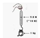
5. The value of g in the British system is 32 ft/sec<sup>2</sup>. The unit of force is pounds. The unit of mass is the slug. Use your weight in pounds to calculate your mass in units of slugs. **PSYW**
